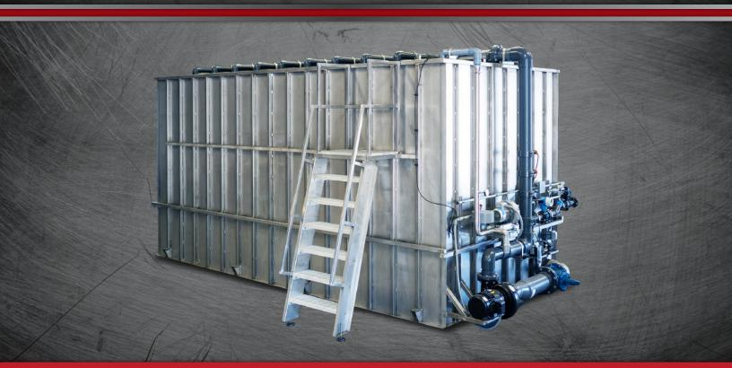
The PRIMEPAC<sup>™</sup> package wastewater treatment plant utilizes the attached growth treatment process to reduce Biochemical Oxygen Demand (BOD) an average of 70%. This system is designed to treat process wastewater in an energy efficient manner by utilizing fixed film growth and growing naturally occurring anaerobic and aerobic bacteria on the same media.
