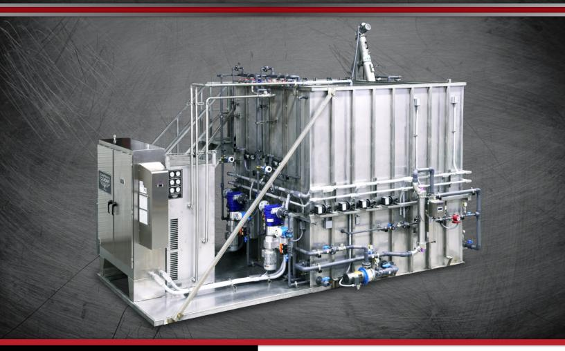
Cloacina's MEMPAC-X is a cost-effective treatment solution designed for low flow domestic applications with stringent discharge requirements. The base unit can treat up to 20,000 gallons per day and is designed to be easily expanded to treat up to 45,000 gallons per day with the incorporation of additional Cloacina or Client-supplied external tanks. This system can reclaim 100% of the treated effluent for irrigation and sanitation purposes and has expedited construction and delivery timelines.
