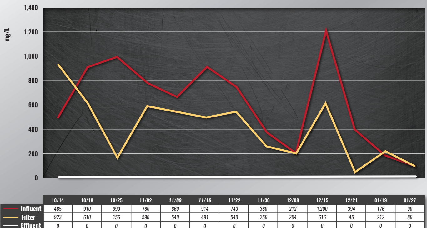
Graph illustrates Total Suspended Solids(TSS) reduction by the MEMPAC-I from system start-up through 2016 harvest
