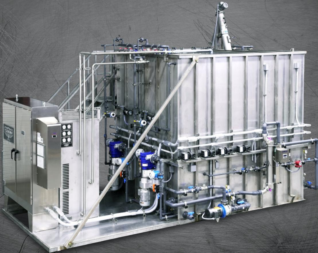
Cloacina's MEMPAC-X is a cost-effective treatment solution designed for low flow domestic applications with stringent discharge requirements. The base unit can treat up to 20,000 gallons per day and is designed to be easily expanded to treat up to 45,000 gallons per day with the incorporation of additional Cloacina or Client-supplied external tanks. This system can reclaim 100% of the treated effluent for irrigation and sanitation purposes and has expedited construction and delivery timelines.
